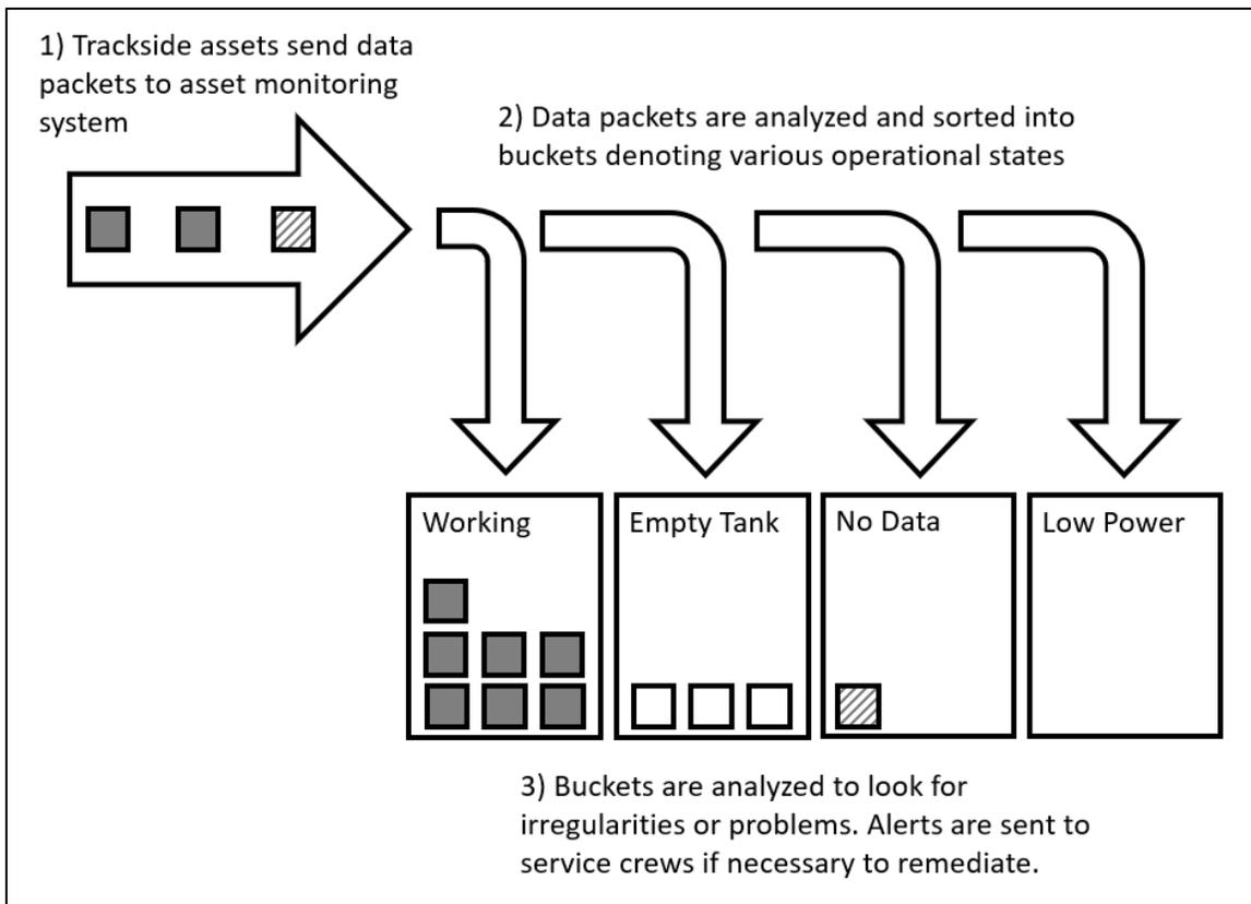
**FIGURE 1: State of each asset (trackside system) is continuously monitored and categorized**
